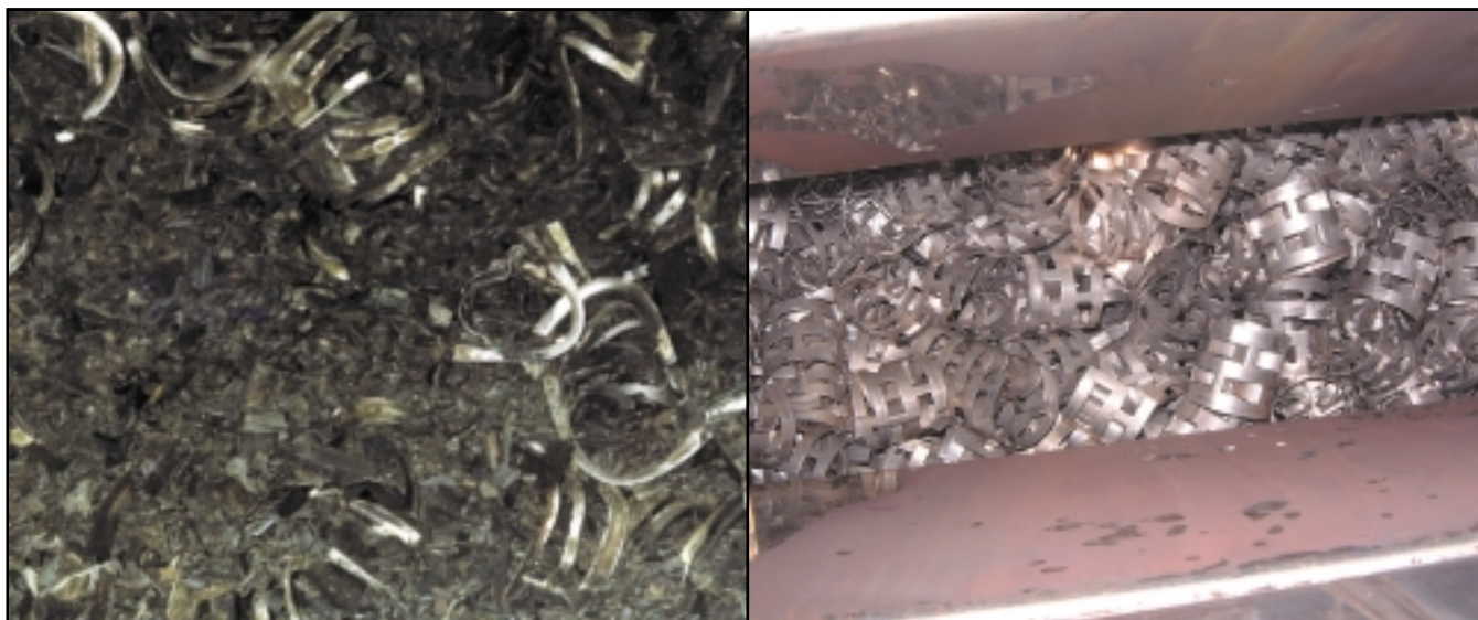
Stripper packing prior to GAS/SPEC CS-2000 (above left) and with GAS/SPEC CS-2000 (above right).
