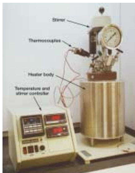
Fig. 1. The testing apparatus showing the temperature and mixer controller.
