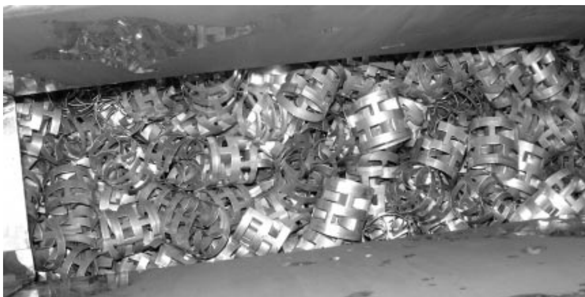
Fig. 2 - Tower Packing after a full year of Service with GAS/SPEC CS-2000.
